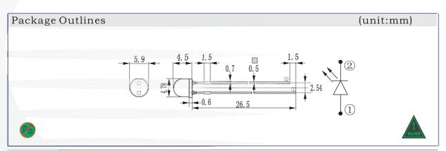
Remark: 1. All dimensions are in millimeters, tolerance is 0.25mm unless otherwise noted. 2. Above specification is measured by CHANGLI's test instrument and may be changed without notice. 3. Supplier will reserve authority on material change for above specification.
