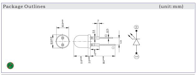
Remark: 1. "\(\triangle^{n}\) represents Internal Circuit Feature: A. C. E...Common Cathode, B. D. F...Common Anode.
