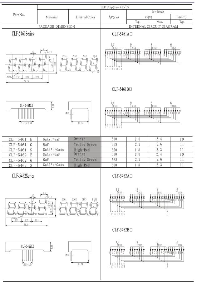
"△" represents Internal Circuit Feature: A、C、E…Common Cathode, B、D、F…Common Anode.
